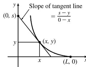
Thus,  $s = y - x \frac{dy}{dx} \Rightarrow \frac{ds}{dx} = \frac{dy}{dx} - \left( x \frac{d^2y}{dx^2} + 1 \frac{dy}{dx} \right) = -x \frac{d^2y}{dx^2}$ . Equating the two expressions for  $\frac{ds}{dx}$
